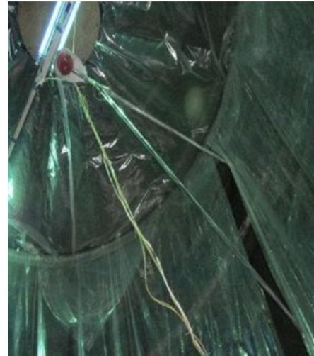
Fig. 2. Large cloud chamber. On the left – diagram of the arrangement of equipment and devices, on the right – example of the arrangement of a source of ultraviolet radiation for ozone generating.
