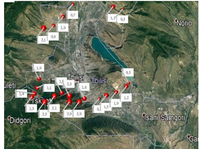
Fig. 4. Places of the falling hailstones and calculated values of their maximum size on the earth's surface in Tbilisi during two hail processes on 10 June 2017 (numbers below - sizes of hailstones, cm)
